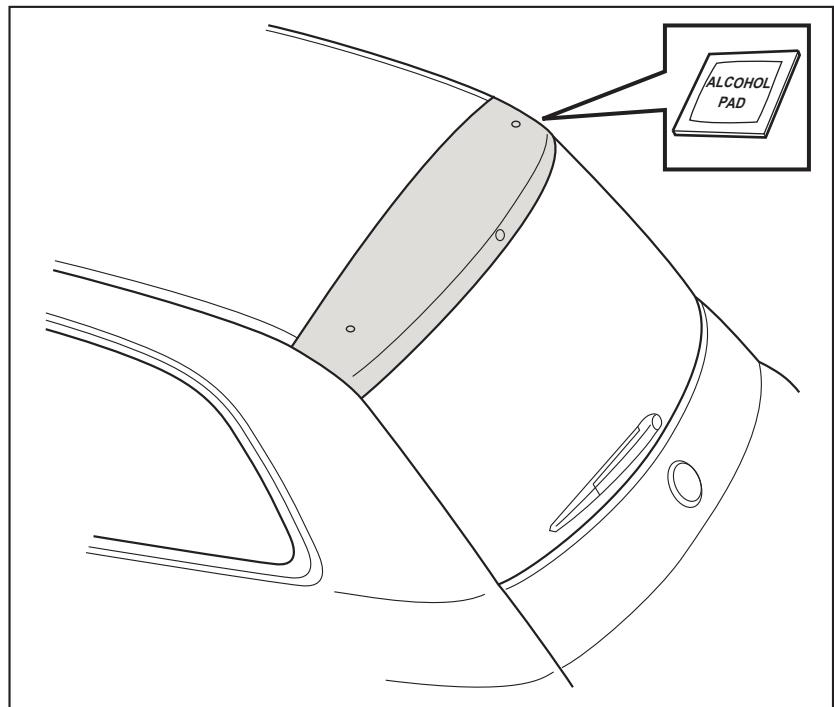
5. Place the spoiler upside down on a secure work surface. Remove the two (2) inner mounting clips by sliding them towards the center of the spoiler until they unsnap from the mounting slots. These clips will not be reused. Use alcohol to clean the grooved area all around the inside of the spoiler as indicated. Once the alcohol has dried, apply a thin coat of black primer to this same area. Allow to dry thoroughly. Be sure to apply urethane adhesive within one (1) hour once primer is dry.
