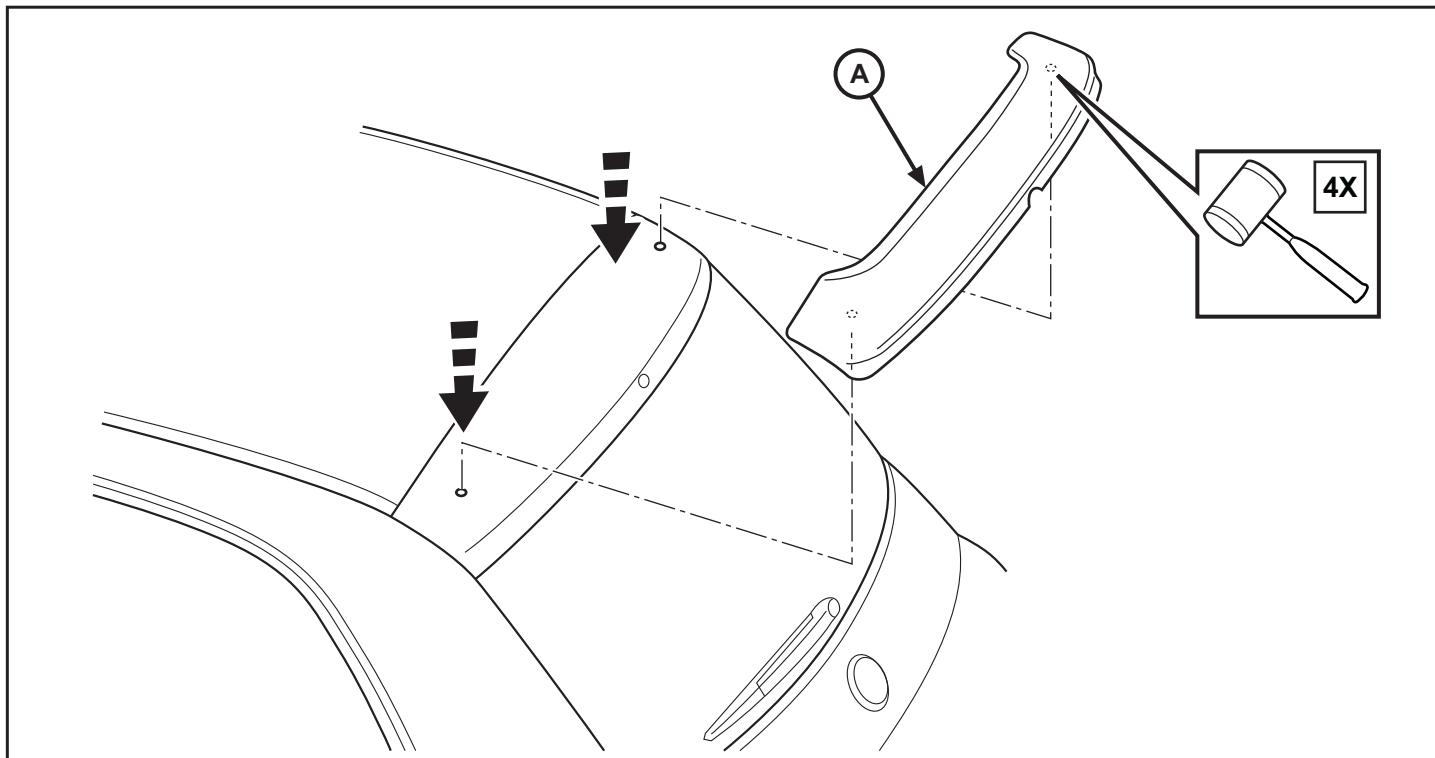
8. Open the hatch and secure the spoiler by wrapping low-tack tape around the left and right edges as shown. Close the hatch and apply tape along the leading edge of the spoiler as shown.
