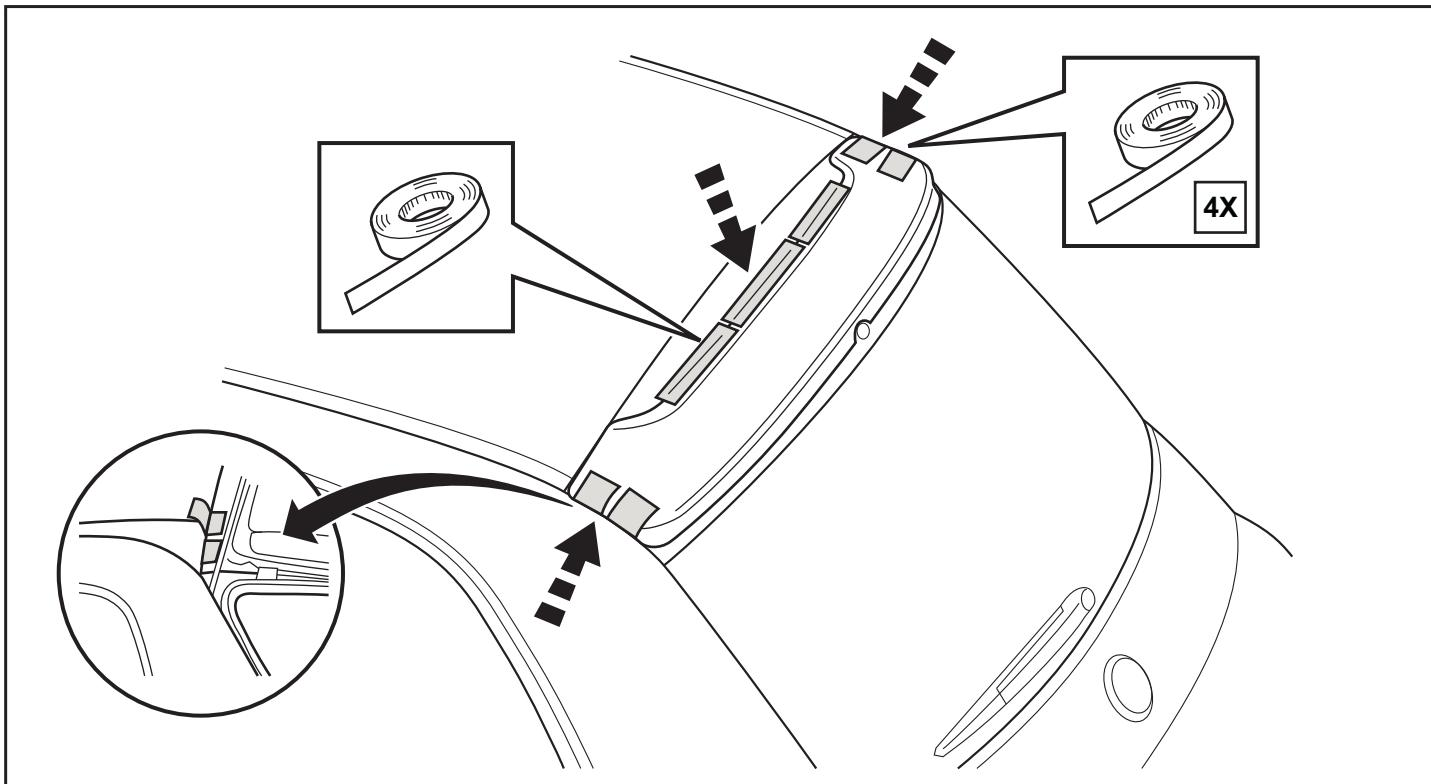
9. Using a roller or hand, apply pressure with 15 lbs force evenly back and forth across the top of the spoiler to help seat the adhesive.
