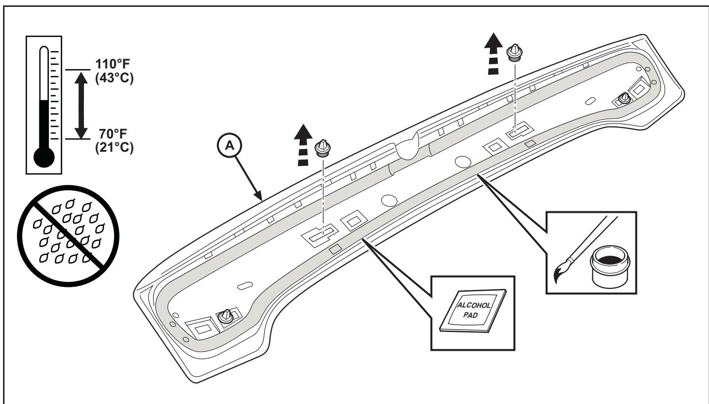
6. Apply a continuous bead of urethane adhesive MS-CD927 to the inner grooved surface of the spoiler. Begin at the point shown and work the adhesive around clockwise, keeping an even amount of adhesive flowing at all times. Avoid bubbles. To finish, apply four 'buttons' of adhesive in the corners as shown.
