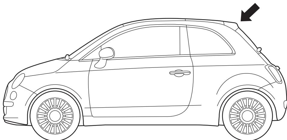
2. Trim out template, position along top of rear hatch and tape into position with low-tack tape. Be sure the forward left and right corners are flush with the corners of the hatch. Mark hole positions with a punch. Remove the template.
