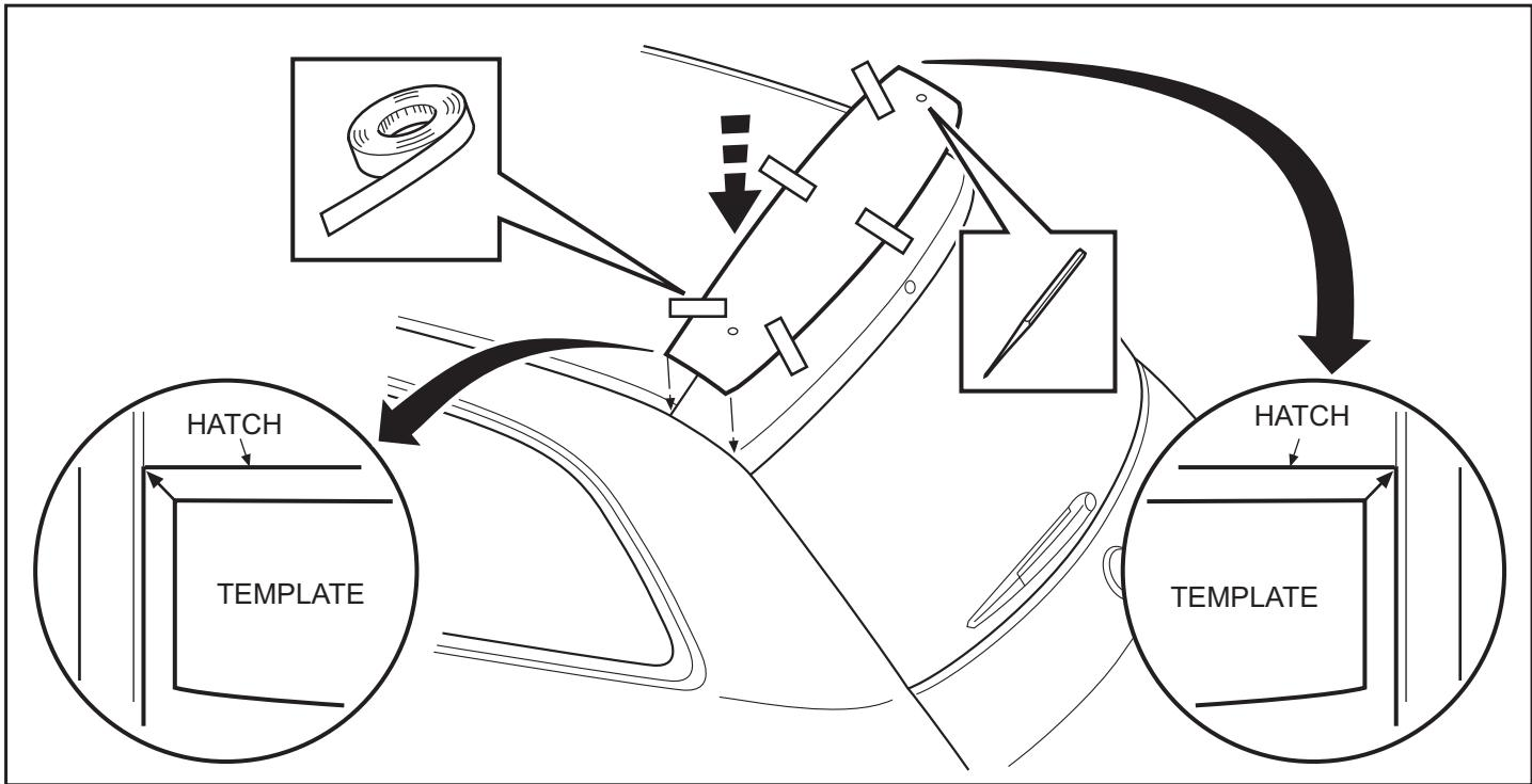
3. Drill two (2) 9.2mm (3/8") holes, one at each marked position. Use a drill stop set to 15mm to avoid drilling through too far. Use a deburring tool to clean each hole. Hold the spoiler in position on the vehicle to check the fit of the holes against the two mounting clips before applying any adhesive.
